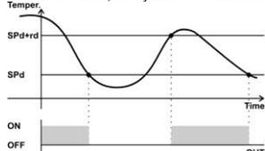
The COOL relay of the slave module activates when temperature is  $t \geq SP + rd$  and turns off when it reaches the set-point temperature **SP**.
